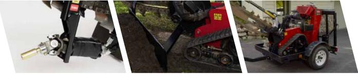
Simplify irrigation and cable installations under driveways and sidewalks with the bore drive head. It can be lowered into the trench to aid in level operation. Backfill open trenches efficiently and finish the job with the backfill blade, which can be installed in less than a minute.
